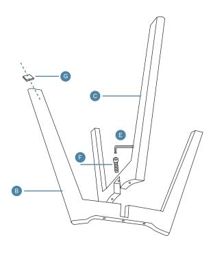
Attach 1 x leg (B) and 1 x leg (C) together as shown and secure with 1 x bolt (B) and 4 x foot pads (G). Tighten with an Allen Key (E).
