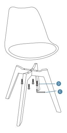
Attach assembled legs to chair as shown and secure with 4  $\times$  bolts (D). Tighten with an Allen Key (E).
